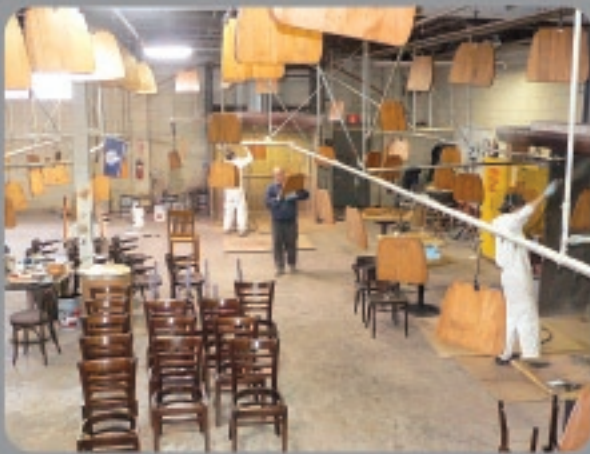
Single conveyor line moves product through finishing process from sanding to staining, lacquer and drying.
