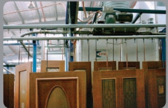
Large wooden doors are conveyed from the finishing line through the assembly process to shipping.
