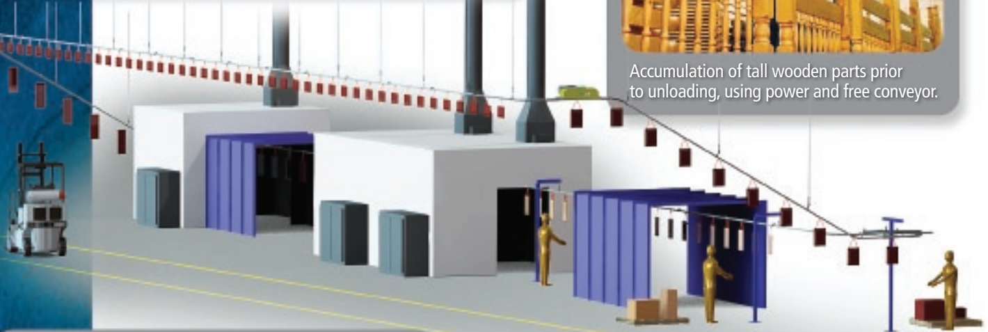
Paint line conveyor moves kitchen cabinets into warmer, unused overhead space for shorter drying time.
