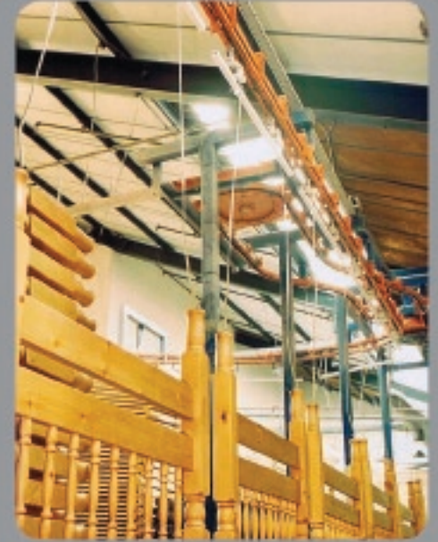
Accumulation of tall wooden parts prior to unloading, using power and free conveyor.
