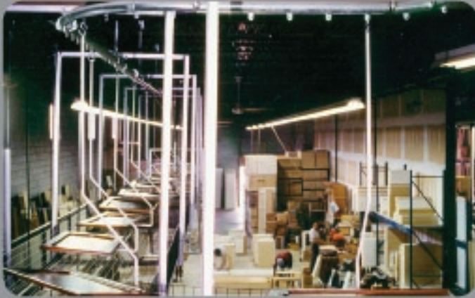
Paint line conveyor moves kitchen cabinets into warmer, unused overhead space for shorter drying time.
