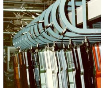
**Powered Over-N-Unders** utilize a standard Unibilt drive to move parts from load to unload. Powered Over-N-Unders are not restricted to straight loop designs. Horizontal turns and vertical curves can be incorporated to bypass aisles and other obstacles.
